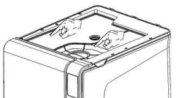
Clean the internal tank surfaces with a soft sponge and a mild detergent solution, then rinse and dry them. Make sure the drain tube is connected to the tank you are cleaning (left tank – grey colored connector; right tank – blue colored connector) to drain the detergent solution.
