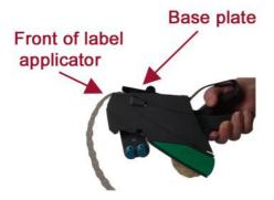
Feed the labels through and out the back of the transport unit (L) until the labels emerge between the tear-off edge (M) and the handle lever (A).
