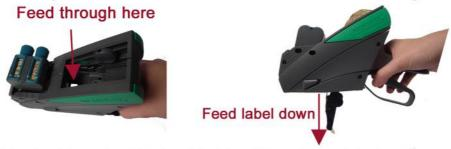
3. Slide the new label roll into the label roll holder (C) until the label core snaps into place. The labels should be placed in the holder with the label side facing up.
